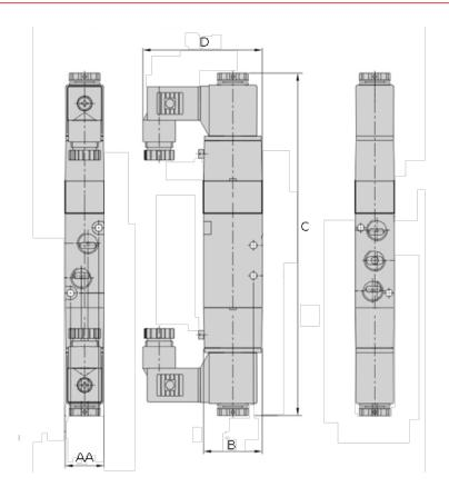
$\begin{array}{lll} \text{AA} & = 18 \\ \text{B} & = 27 \\ \text{C} & = 99.4 \\ \text{d} & = 55.0 \\ \text{Port exit} & = G 1/8" \\ \text{Port supply and blowdown} = G 1/8" \\ \text{Voltage} & = 24 \text{ VAC} \end{array}$
